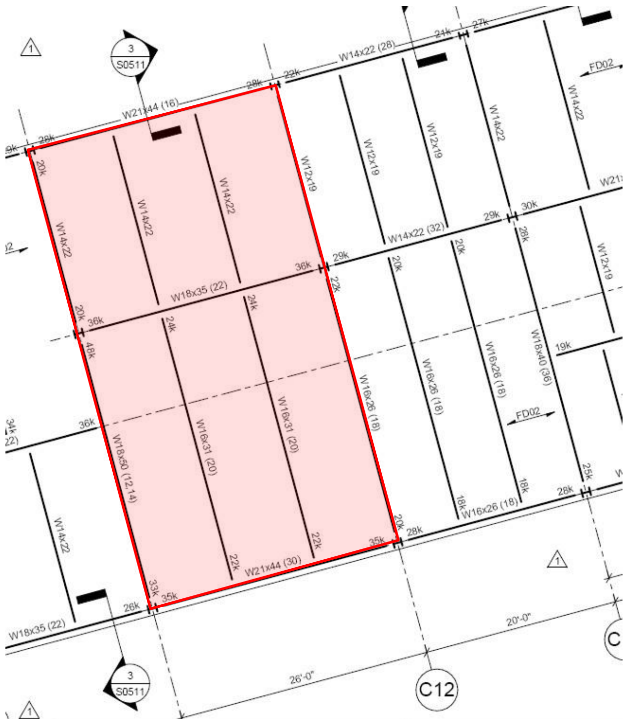
Figure 13: Typical Floor Plan of existing structure with bays used in calculations highlighted. Drawings courtesy of Cannon Design.
